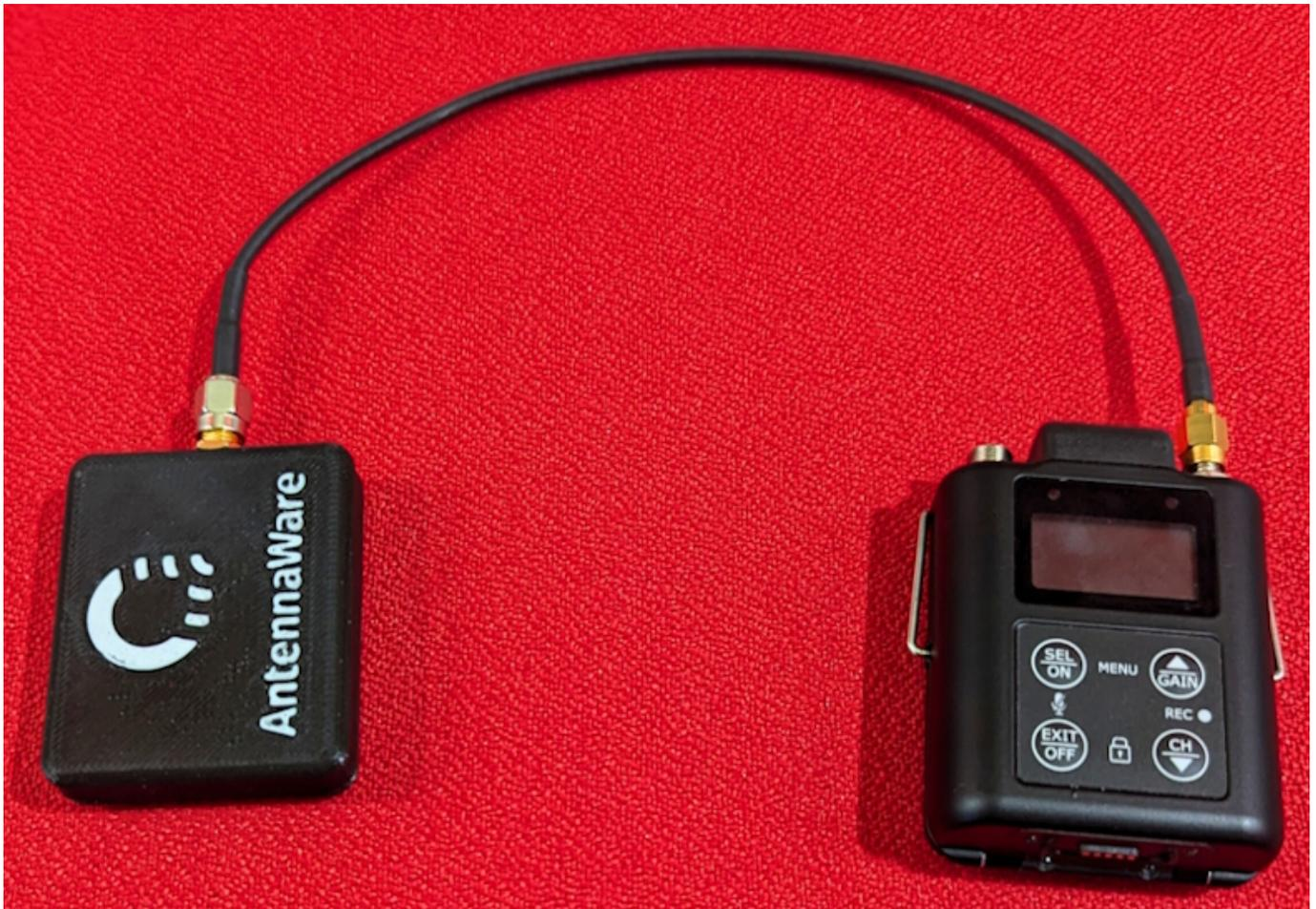
Launched at IBC 2024, the Sub-GHz BodyWave antenna promises notable increases in wireless range and reliability of signal in a form factor designed specifically to be compatible with virtually all bodyworn UHF transmitter packs.
