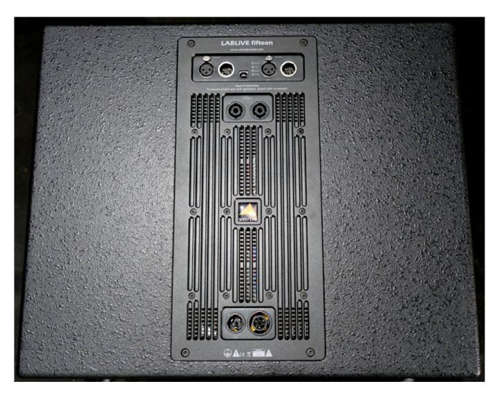
The whole system is driven by an active module which in addition to a user DSP contains three Class D power amplifier channels. The subwoofer is fired with 1,000 watts, while 500 watts are available for two passive tops. A Neutrik True1 fitting supplies the system with the necessary mains voltage. The True 1 plug can also be plugged in and unplugged under load, which is why the active module does not require a dedicated power switch.
