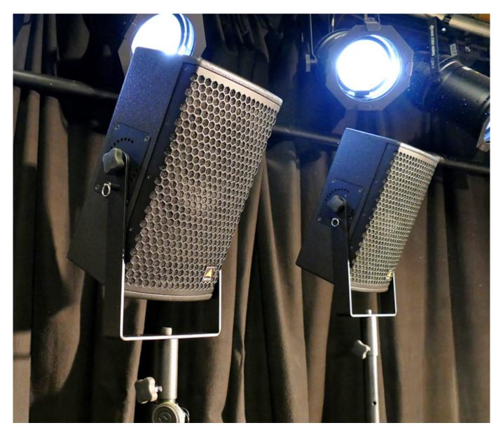
The preferred play partners of the LABLIVE fifteen subwoofer are the tops from the LABRAT series. Our test system is equipped with two LABRAT eight pro tops. The compact tops with 8 "coaxial drivers, as also the subwoofer, come in padded transport bags and sit on spacer rods via two U-brackets with integrated tripod mounts. The form factor of the LABRAT eight pro is very interesting. The housings have a bass reflex opening and a multifunctional housing with a slope for monitor useage.
