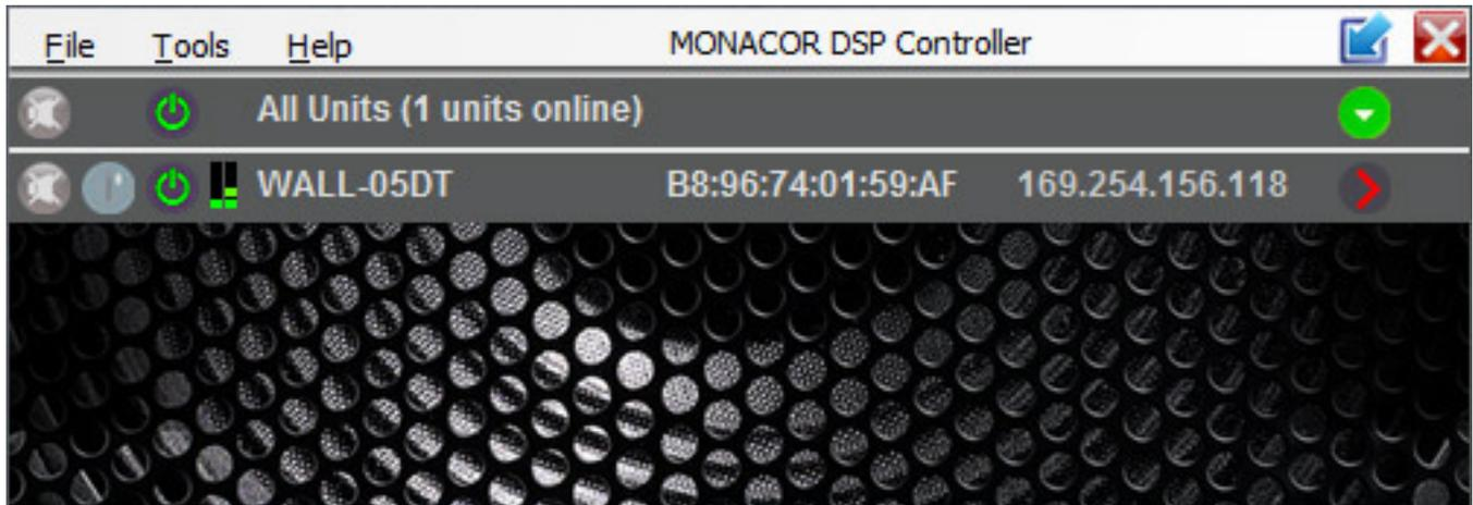
Clicking onto the arrow of the respective network device will open the specific configuration window (see image below).
