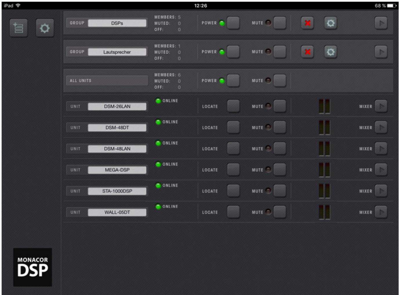
The iPad app provides the same features as the DSP controller software from MONACOR. It is also possible to create device groups. However, the display is designed to match the typical iPad functionality and thus varies slightly from the display of the DSP controller software.
