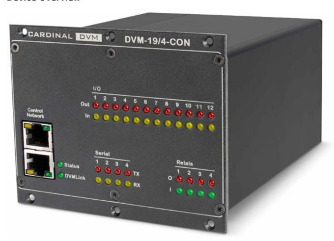
The DVM-194-CON Media Controller is the heart of the DVM 194 series, establishing the connectivity for the media and input devices. Via the web interface instruction macros can be freely defined and entire instruction sequences created. Four RS232 interfaces allow a bi-directional communication with the connected devices – e.g. the checkback signal from the beamer that the lamp needs to be replaced. Via the
