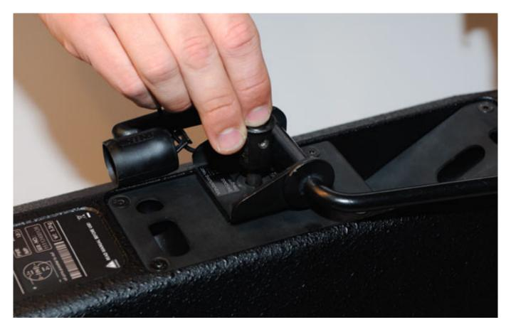
The loudspeaker may be equipped rapidly with an eyebolt or mounted for fixed installation with the M10 threading. Beside the pivoting speaker mount, accessories are the stand socket and the tube clamp as well as a mini TV spigot and a pin joint adapter, e.g. for the fastening of a crossbar. Neumann & Müller designed a different solution for its own application which is available especially for Neumann & Müller.
