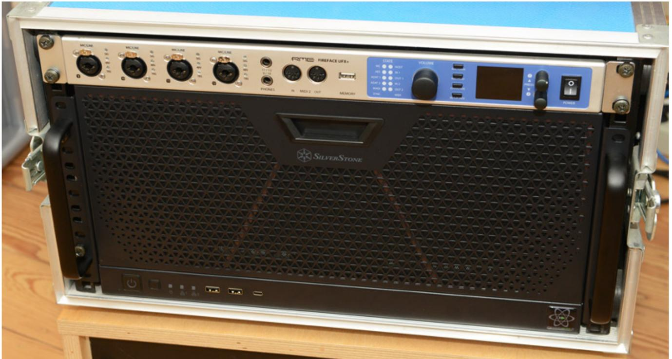
Let us start with the housing. The 19-inch rack brackets on the side are slightly shorter and do not cover the entire 5 U high area. In our rack, it was not possible to use the holes above and below the handle, but this was not a problem, as there are eleven mounting holes on each of the brackets. In contrast to the previous computer, we used a support guide because the weight could be placed in the rack without a support guide for assistance.
