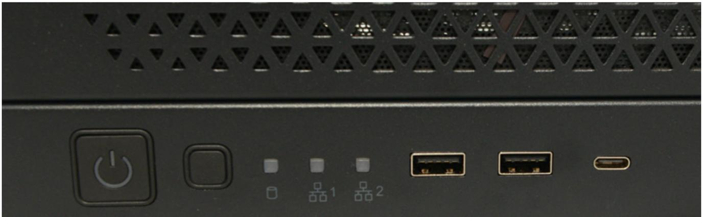
There are only a few operating elements on the front panel. In addition to the on/off button, there is a reset button and status indicators for hard drive activities and networks. There are also two USB-A ports (USB 3.0 with 5 GBit/s) and one USB-C port (USB 3, 5 GBit/s) on the front panel.
