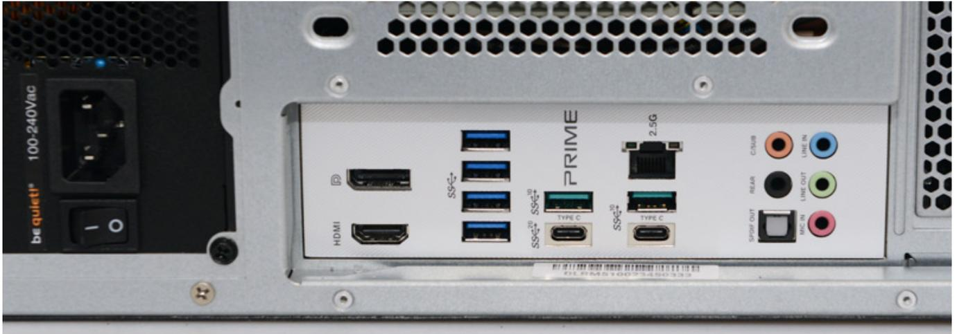
The motherboard's connections also offer a 2.5 GBit/s Ethernet port, as well as six USB-A ports (USB 3.2 Gen 1 and labeled blue with 5 or green with 10 MBit/s) at different speeds and two USB-C ports (USB 3.2 Gen 1 with 10 or 20 MBit/s). A total of 13 USB ports at the back of the entire computer.
