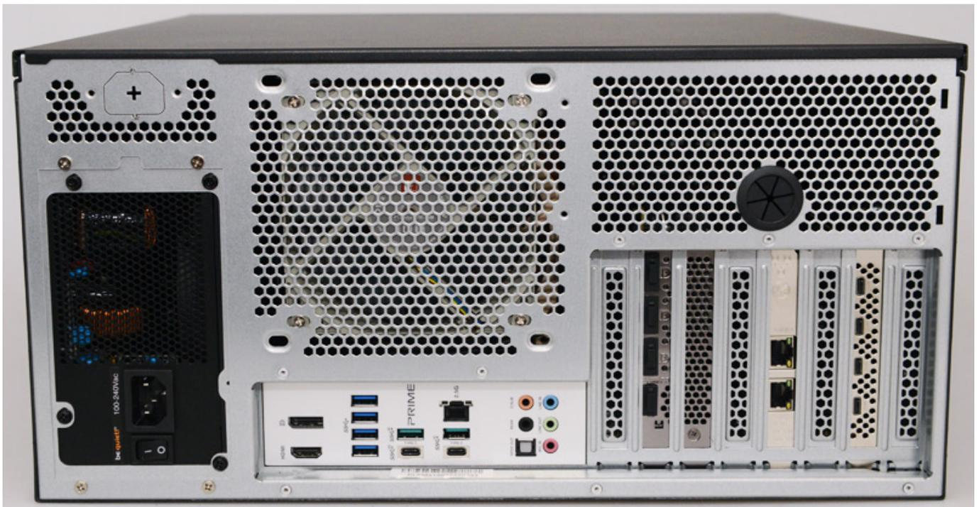
The AudioKern B14 is equipped with a LAN card with two 1-Gigabit Ethernet ports so
