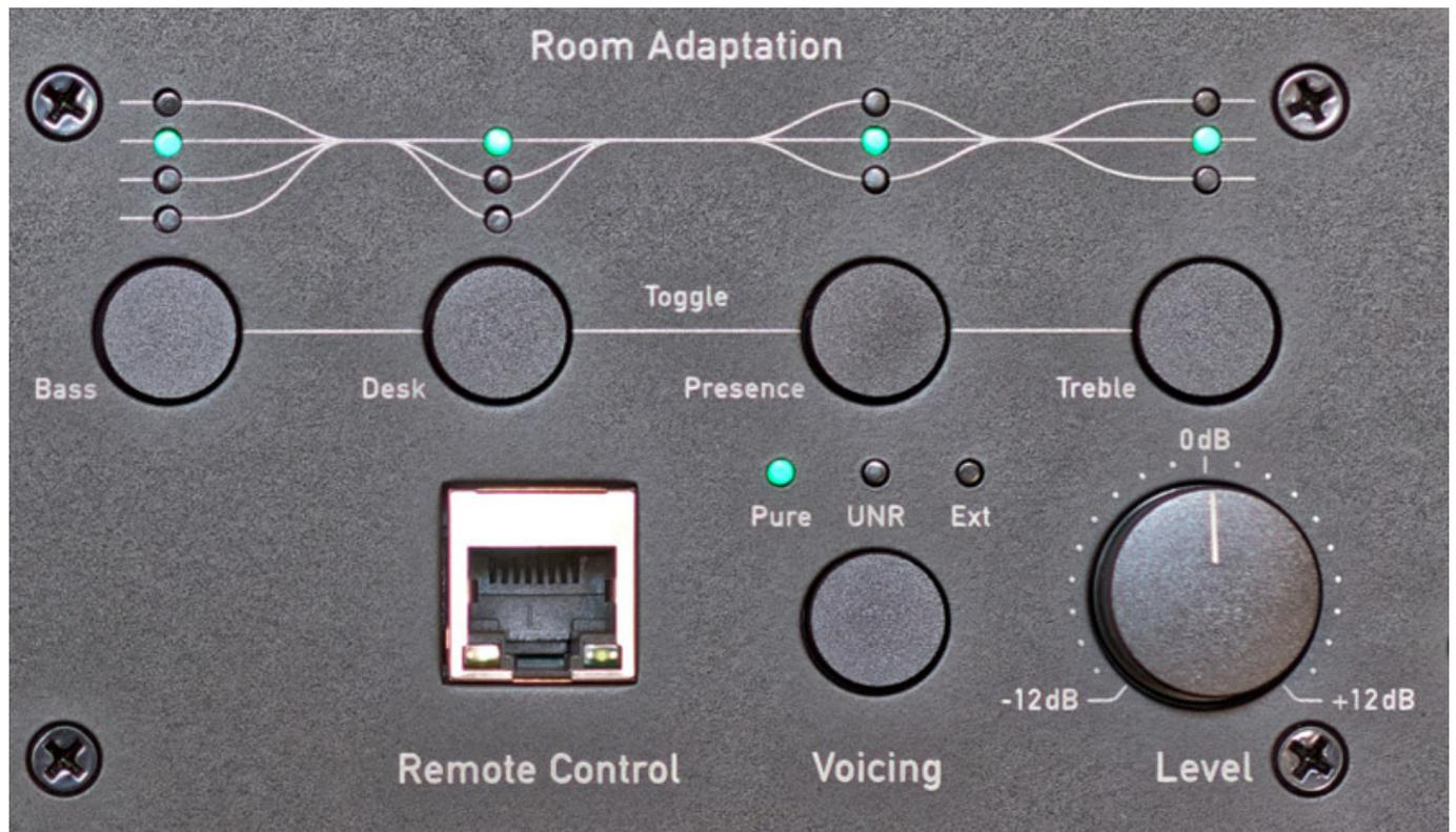
In this context, the "Pure" setting stands for the basic sound tuning of the current A-Series, while "UNR" activates a legacy mode with the classic playback curve of the superseded X-Series, so to speak. The Ext(ern) setting can be used to load a profile created using the SoundID Reference room correction software from Sonarworks. In addition to the obligatory gain control (-12dB to +12dB) and balanced (XLR) and unbalanced input (RCA), the A-Series also has an RJ45 network socket.
