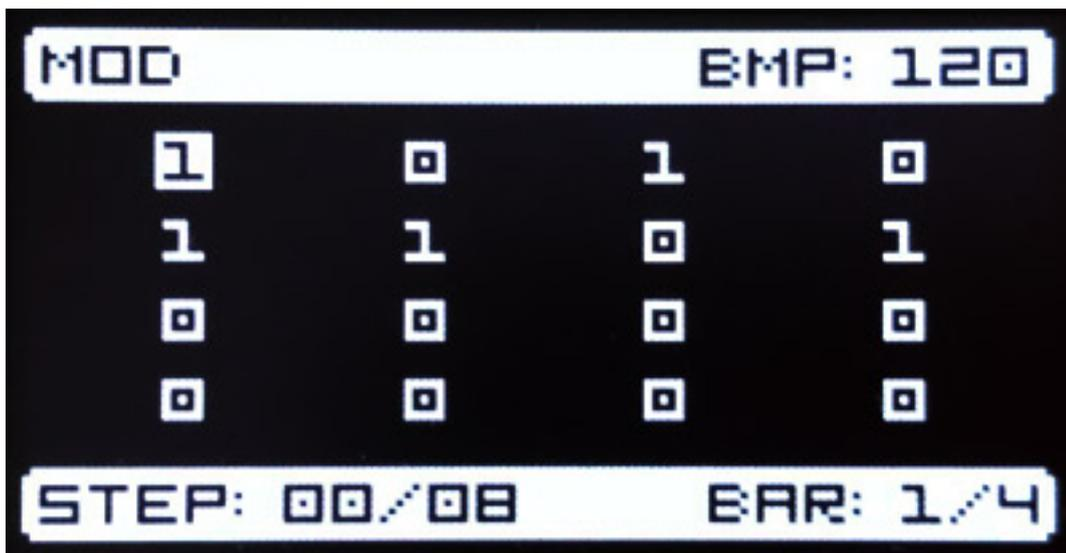
Another very interesting modulation mode is the trigger mode. Every step features a trigger impulse configured (turned on / off) by pressing on the corresponding encoder, enabling a tighter integration with drum and percussion modules. The flexibility is slightly hampered by the limited range of lock divisors but sufficient for
