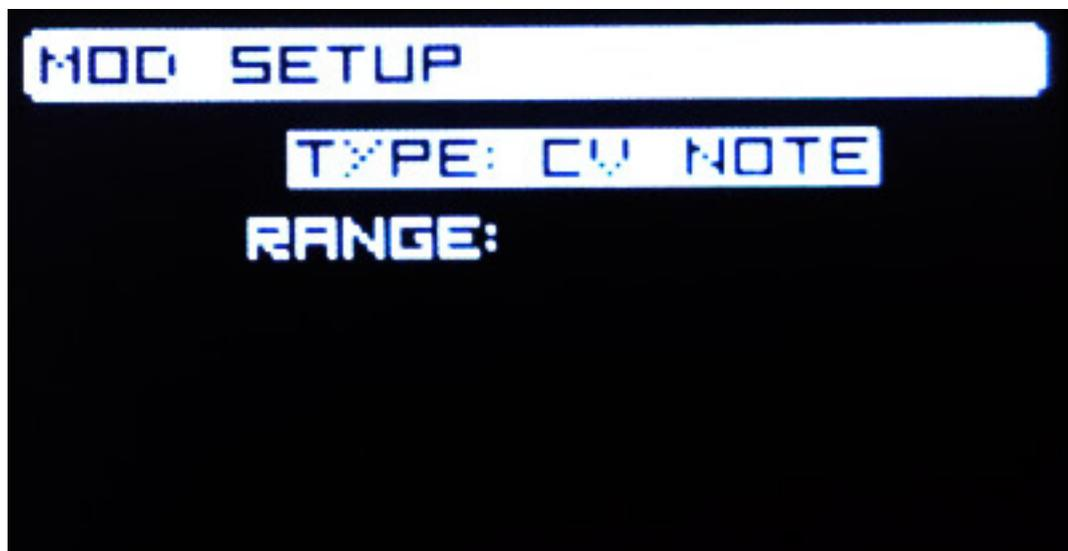
Let's have a look at the modulation output that has a multitude of uses. Pressing SETUP+MODE accesses the configuration dialog.
