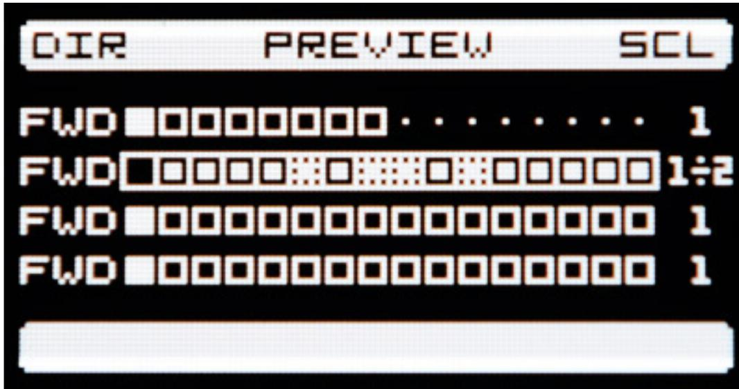
With the key combination SHIFT + DRCTN RANGE a 16 step overview of all four tracks appear including playback mode and clock divider/multiplier.
