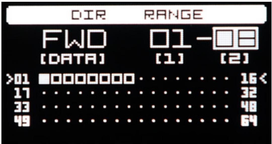
DRCTN RANGE accesses a dialog that controls the playback-direction of the current pattern: forwards, backwards, ping-pong and random. Also the playback range (start and end point) can be set by pressing one of the 16 encoders.
