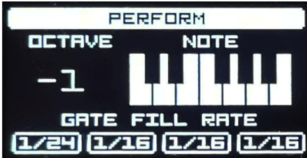
In the 1.0 release there is a perform dialog available for transposing by the first 12 encoders and rolls can be filled by pressing the encoders 13 until 16. The roll rate can be adjusted by these four encoders.
