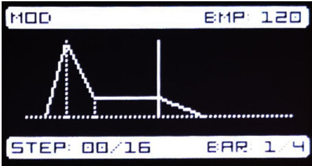
It is possible to output a defined voltage or a voltage corresponding to a note. There are also modes to output AD, ASR or ADSR envelopes.
