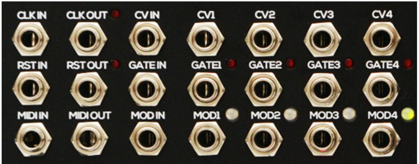
Let's have a look at the connections first. On the right hand side you will find the outputs for CV, gate and modulation voltages for the four tracks. To the left there is one input each for CV, gate and modulation. The Black Sequencer also sports inputs for clock, reset, MIDI in- and output, all as 1/4" (3,5mm) TS sockets.
