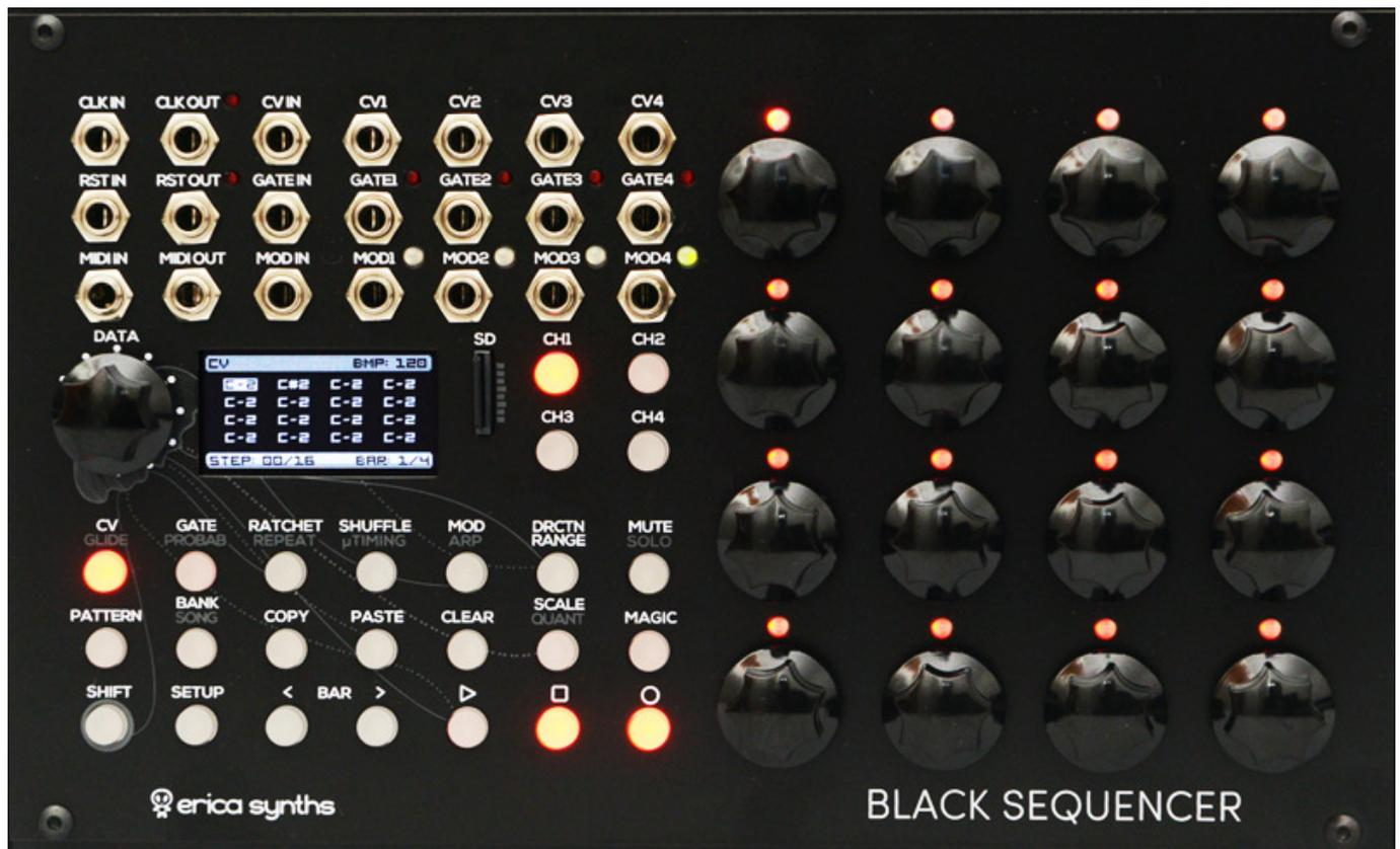
Power consumption tops out at 114mA at +12V and 24mA at -12V. This is quite moderate compared to other sequencer modules. +5V is not required.
