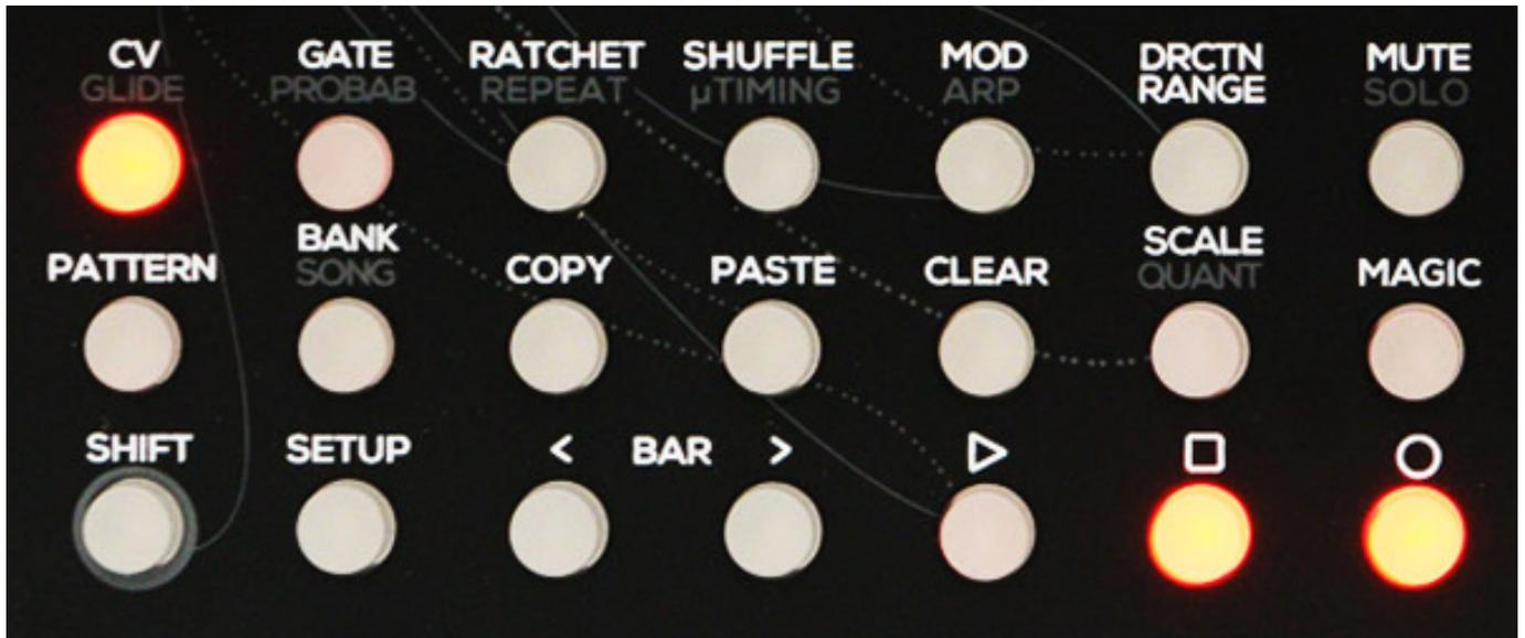
The lower row offers access to relevant system functions such as configuration, starting, stopping and saving the current configuration. Whenever a pattern has been changed the record-key denoted by a circle blinks. By the way, all buttons are illuminated by red LED's as indicators. So much for the basic handling of the sequencer.
