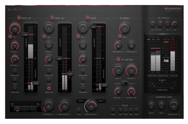
Brainworx, a part of Native Instruments, today announced the release of bx\_XL V3, a mid/side mastering limiter plugin that delivers ultra-loud masters with XL saturation. By utilizing the mid/side technology from Brainworx's groundbreaking bx\_digital EQ, the bx\_XL V3 empowers mastering engineers to achieve loud masters without sacrificing clarity. The mid channel is split into two bands, allowing for control over three individual channels – mid-low, mid-high, and side.
