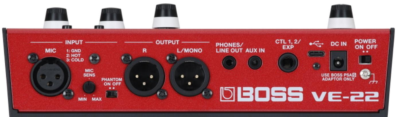
The VE-22 provides an XLR input and integrated preamp for a professional stage microphone, plus phantom power for high-end condenser types. A high/low gain switch, rear-panel sensitivity knob, and level meter enable the user to optimize the input signal for nearly any mic. USB-C, an analog aux input, and a headphone jack support a variety of vocal activities, including daily practice, computer recording, music playback from a smartphone, and livestreaming on social media.
