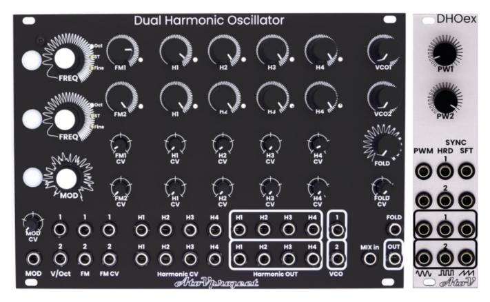
The AtoVproject DHO or Dual Harmonic Oscillator is a n ovel take on the complex oscillator concept. It is an analog oscillator with digital control and also the first Eurorack module to feature haptic feedback. Each analog oscillator generates four octaves of triangle waves and modulates each other using through-zero frequency modulation. All of this is channeled through a four-stage diode wavefolder.
