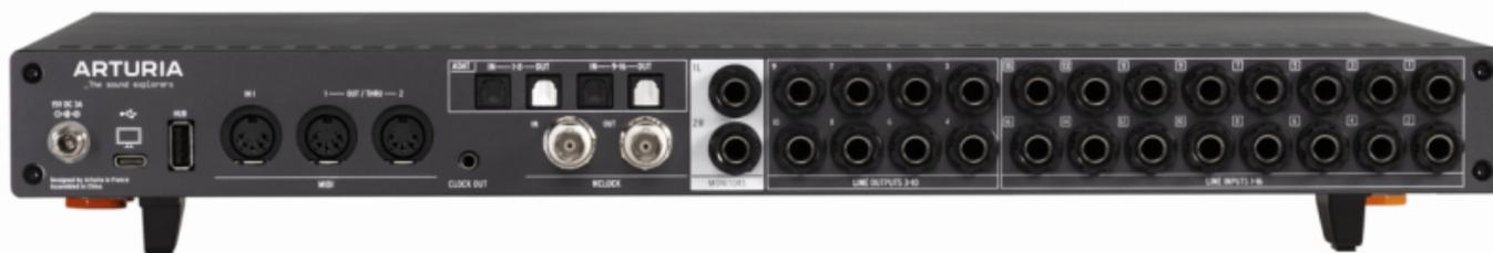
Users can control settings via the built-in controls or the included software, configure it for desktop or rackmount operation, and even connect high-impedance headphones. Save configurations & mix settings as presets, control modular gear with DC-coupled outputs, use the Reamp feature for versatile guitar tracking, and connect extra USB devices with class-compliant connections.
