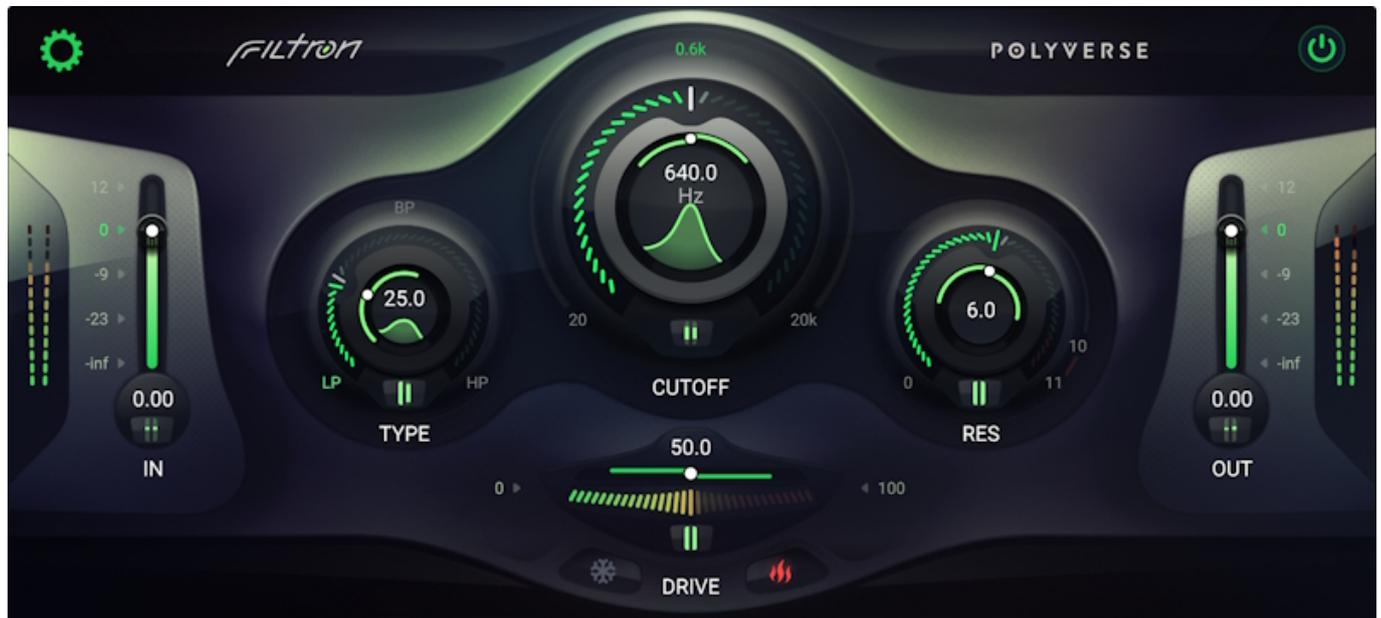
Filtron is a 12dB state variable filter that can smoothly transition between lowpass, bandpass, and highpass. It is capable of self-oscillation with resonance levels that can reach up to 11. Filtron also features a fat sounding internal saturation algorithm and a sizzly post overdrive with two modes to choose from: cold and hot.
