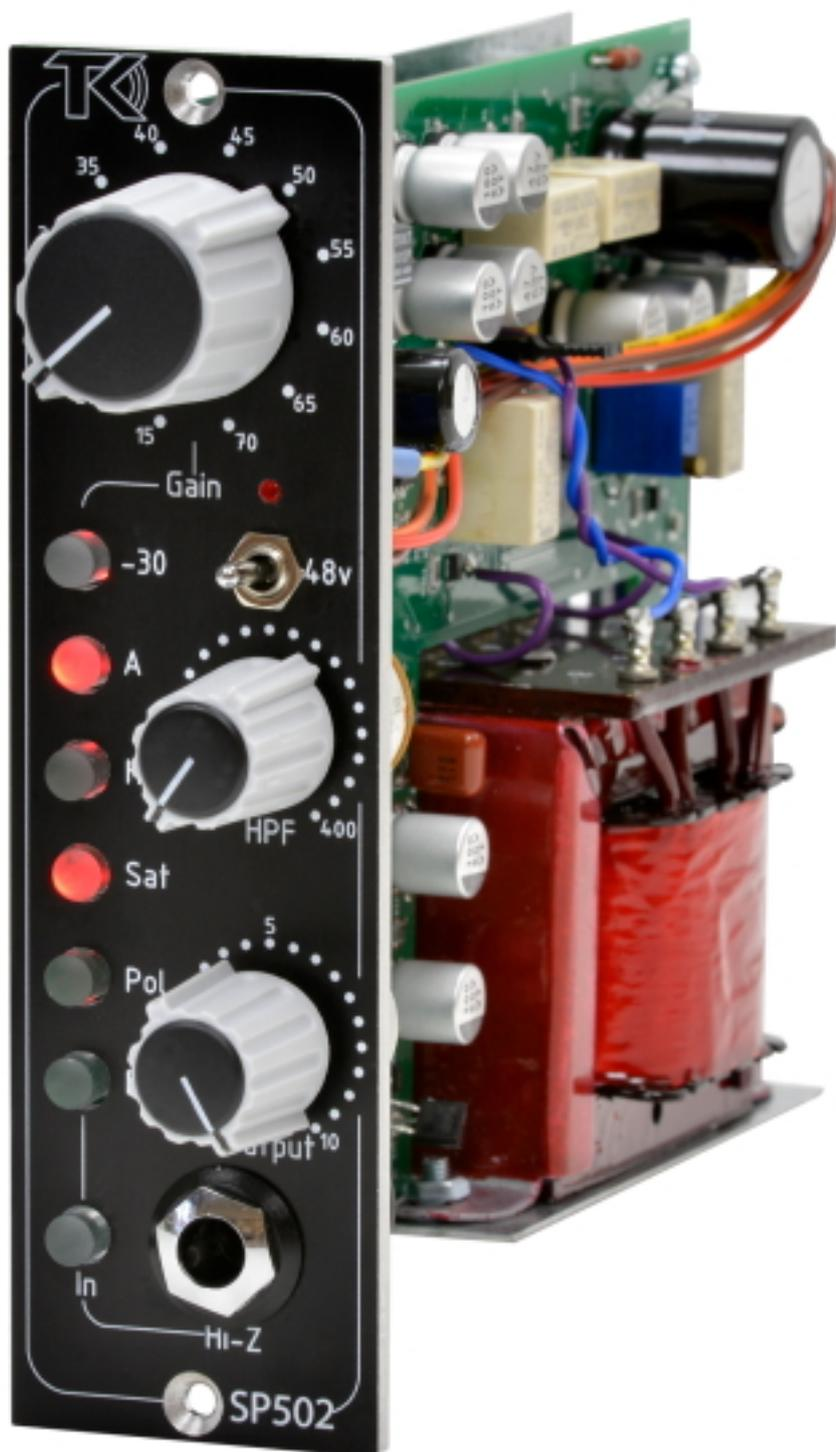
SP502 is a new single slot 500-series preamp with a unique hybrid design including both vintage and modern circuits. A new transformerless input stage forms a clean and transparent front-end, together with the two selectable output stages you can get the low mid punch and thick sound associated with British Class A from the early 70's as well as a more modern clean tone from the 80's and 90's.
