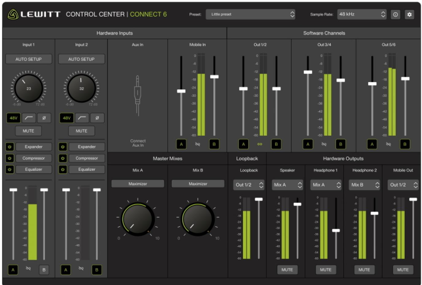
For example, Mix A could be used for personal monitoring while Mix B is being sent wherever you need it, be it your DAW, a streaming software, or a virtual meeting. You can even send your mix to applications on your mobile device. Both mix outputs feature a one-knob Maximizer to ensure that your mixes always have the optimal loudness level.
