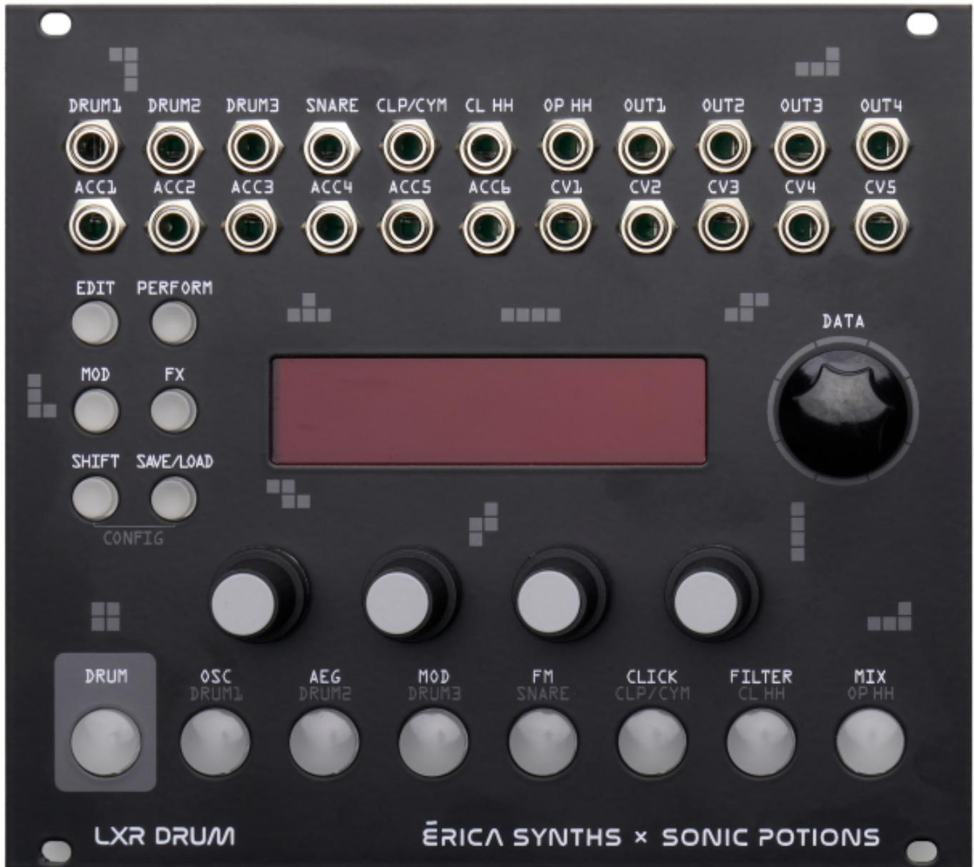
LXR eurorack module is a compact and great-sounding percussion synthesizer based on the sound engine of the LXR-02 drum machine. While retaining the core interface of the LXR-02, this module adds the essential eurorack ingredient - assignable CV control over parameters and many more tweaks in the user interface for better integration in any eurorack system.
