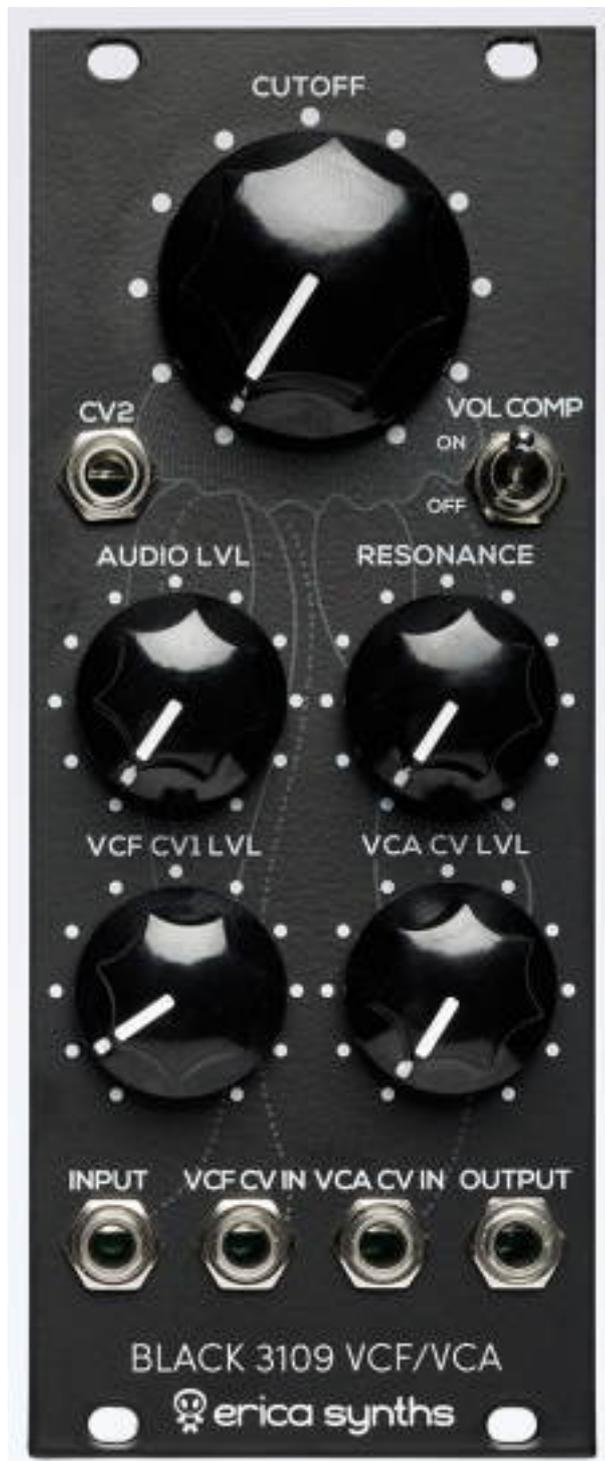
The Erica Synths Black 3109 VCF/VCA is a lowpass filter and voltage-controlled amplifier combo built around the AS3109 VCF integrated circuit, a contemporary version of the IR3109 chip, found on vintage Roland synths such as the Jupiter series, Juno series and the SH-101.
