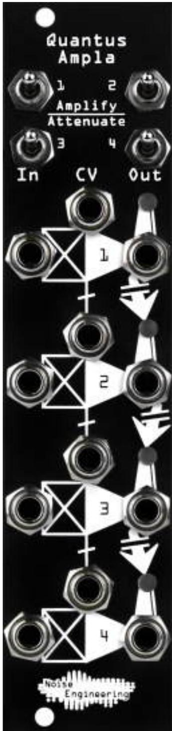
Quantus Ampla is a compact four-channel VCA. But it's not just any VCA: with some unique normalizing, mixing, and CV options, and a bit of NE flair, you can use it for tons of stuff. From the top, each channel has two independent modes: Amplify, which gives you normal VCA response, and Attenuate, which makes the VCAs close instead of open in response to positive CV. The CV inputs are circularly normalised, so
