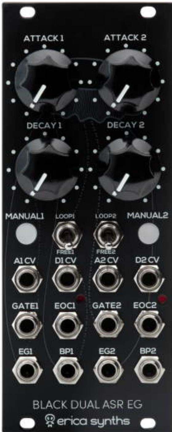
The Black Dual ASR EG is a versatile, full analogue looping AD/ASR envelope generator with voltage control over attack and release times, that can also be used as low frequency oscillator with manually and voltage controlled shape and rate. It has two identical parts, each featuring all typical envelope generator controls and bonus features - the end of the cycle output and bi-polar LFO output. When in loop
