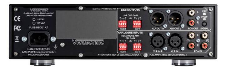
The Violectric HPA V550 is built by hand in the company's own manufacture in Constance. Violectric uses only top-shelf components to suit the refined circuits. Both volume and balance are set via Alps RK 27 potentiometers – except in the PRO version, which employs a 256-step reed relay circuit for the volume. The black anodised housing is topped off by an 8-mm aluminium front plate. Special circuits protect the precious headphones from DC voltage and overload.
