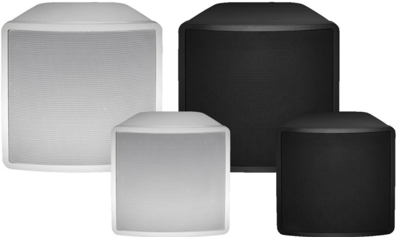
The speakers of the new SL series (stadium speakers) from MONACOR are equipped with 20 cm or 30 cm coaxial horn speakers. With a maximum rated SPL of up to 122.5 dB (sound pressure level: 99.6 dB/W/m), they deliver your messages clearly to the recipient, even across great distances. The SL series features a frequency range of 85 Hz - 19 kHz and is quite capable of also providing pleasant background music.
