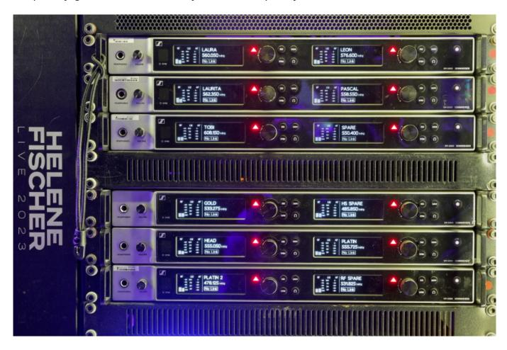
On the "Rausch" tour, the Sennheiser Wireless Systems Manager provided all the important information for operating the wireless systems at a glance. For the battery packs, two Sennheiser L 6000 charging stations were available, each with their own slots in the rack, and these were also connected to the Wireless Systems Manager.
