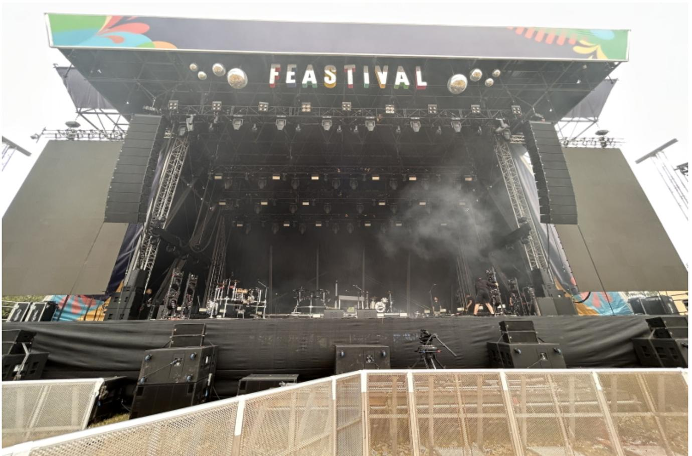
WPL was driven in 2-box resolution from Martin Audio's process-controlled multi-channel iKON amps, and by using Martin Audio's new DX4.0 dedicated system controller, they were able to place the legacy W8LC on the same network, allowing full system control from a single point. A further eight W8LM along the stage lip provided front fills and 12 x XE500 wedges were available to provide additional stage energy. Also providing premium stage fills on each side were a pair of TORUS
