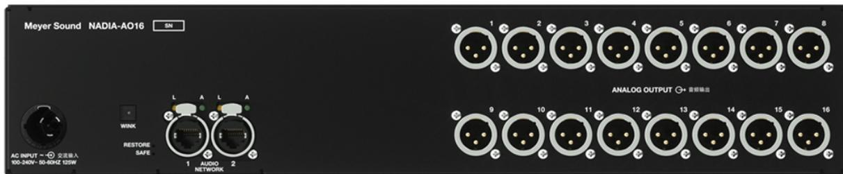
NADIA is an integrated, network-based digital audio processing and distribution platform that will power future installations of Constellation® by Meyer Sound. When incorporated into new Constellation installations, in addition to the processing power and inputs reserved for active acoustics, NADIA also provides separate inputs, processing, and matrixing to enable Spacemap Go spatial sound with no performance compromises for either function.
