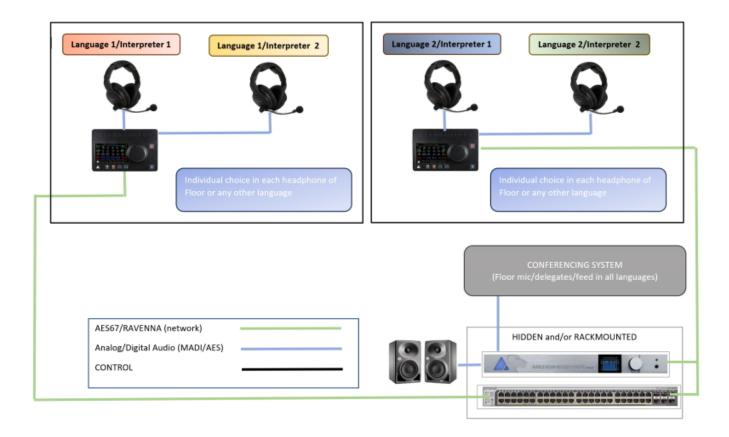
All Anubis are network-interconnected (AES67/ST2110) so that every audio stream can be made available on any Anubis. A Hapi Mk II (AD/DA, Madi, AES/EBU converter) is used as an in/out point with all standard formats to connect to the existing console, PA or conferencing system. One key benefit of this interpretation solution is that it can be remote-controlled via VPN and the IP address of each Anubis.
