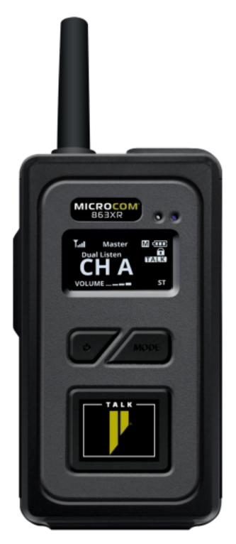
Pliant Technologies announces the latest addition to its MicroCom family of products with the new MicroCom 863XR wireless beltpack. This product is designed for use in Europe as it operates in the 863-865 MHz ISM band, which allows for unlicensed use in most European countries. The 863XR features excellent range, two intercom channels and the capability to support up to six full-duplex users with unlimited
