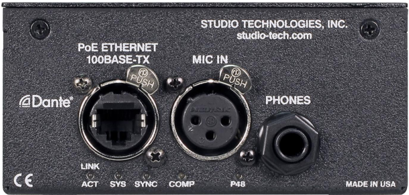
Set up and operation of the Model 203 is simple. An etherCON RJ45 jack is used to interconnect with a standard twisted-pair Ethernet port associated with a PoE-enabled network switch. This connection provides both power and bidirectional digital audio. A broadcast headset or handheld ("stick") microphone can be directly connected to the unit's 3-pin XLR microphone input connector. A 1/4-inch 3-conductor (stereo) jack is used to connect to selected headset, headphones, or an earpiece.
