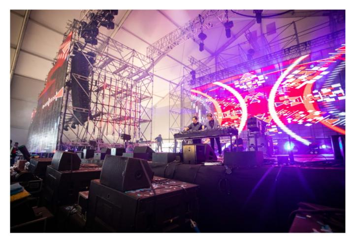
Stage 8 came alive as Paradise on the Friday, transforming into Trick on the Saturday and Solid Grooves on the Sunday. This stage was designed as a unique self-supporting, eight-leg truss structure, from which a WPL PA was flown. The upstage goalposts (left and right) supported WPL, and delays consisted of two hangs of eight WPS, were flown from the last goalposts of the truss structure.
