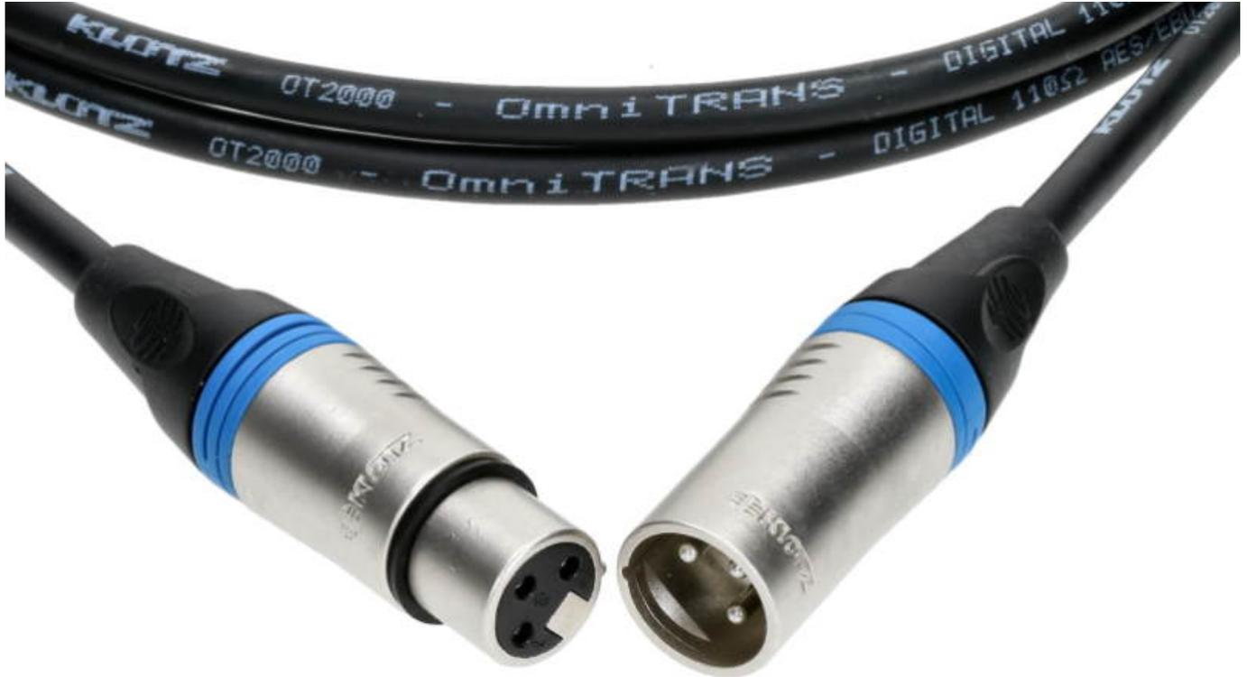
In addition to the successful Pro DMX cables of the LX-5X series with XLR 5 p. connectors, KLOTZ now offers these cable series alternatively with XLR 3 p. connectors (LX-3X). For the LX series, KLOTZ uses only high-quality digital cables with an exact characteristic impedance of 110 ohms.
