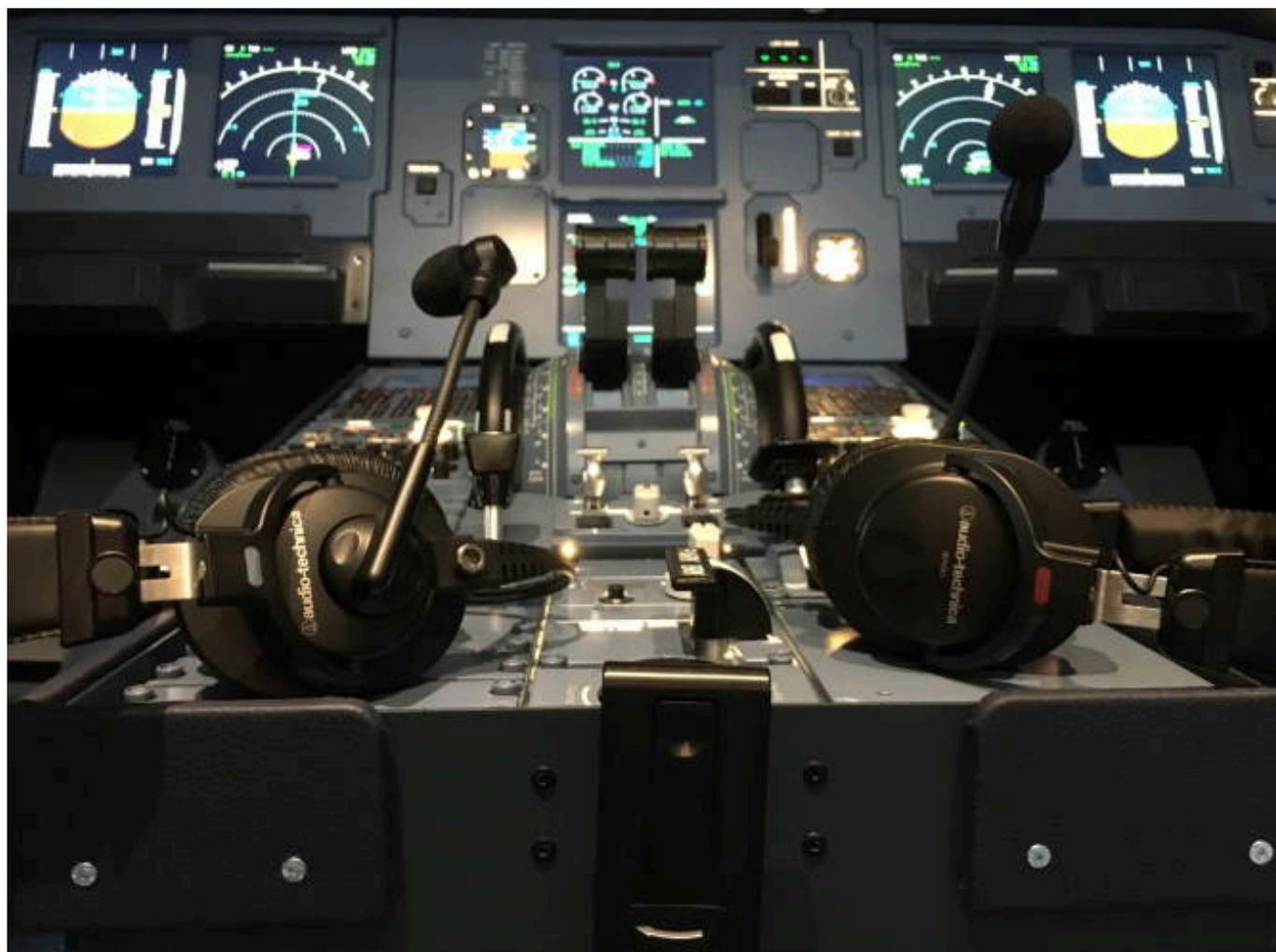
The BPHS1 also provides a similar look and feel to conventional aircraft headsets and allows the microphone and connection cable to be oriented on the right or left side. This is beneficial for the simulators as the connection for the captain/commander comes from the left, and from the right for the first officer, so the versatile positioning of the microphone and connecting wiring avoids cables crossing in front of or behind the head.
