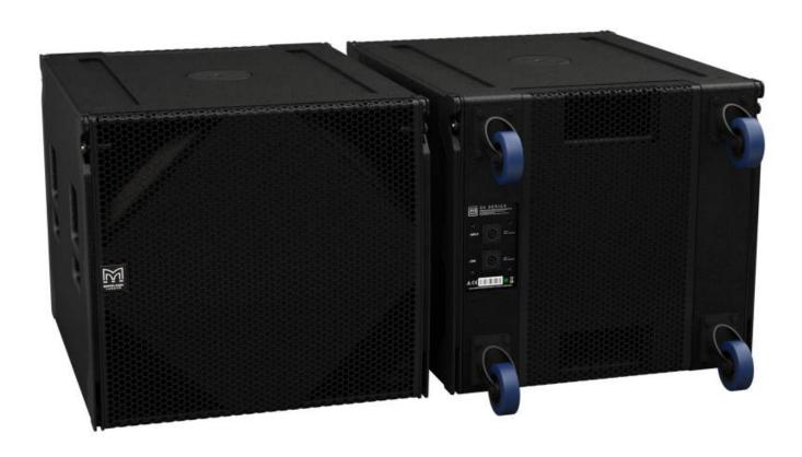
The SXC115 follows similar principles and contains a 15" (380mm) front facing driver and 12" (300mm) rear facing driver, each driven, again, independently by separate amplifier channels and DSP. Each driver, similarly, has its own chamber with optimised bass reflex porting. It is the perfect accompaniment to WPM or alternatively can be used with a pole mount for Martin Audio point source loudspeakers.
