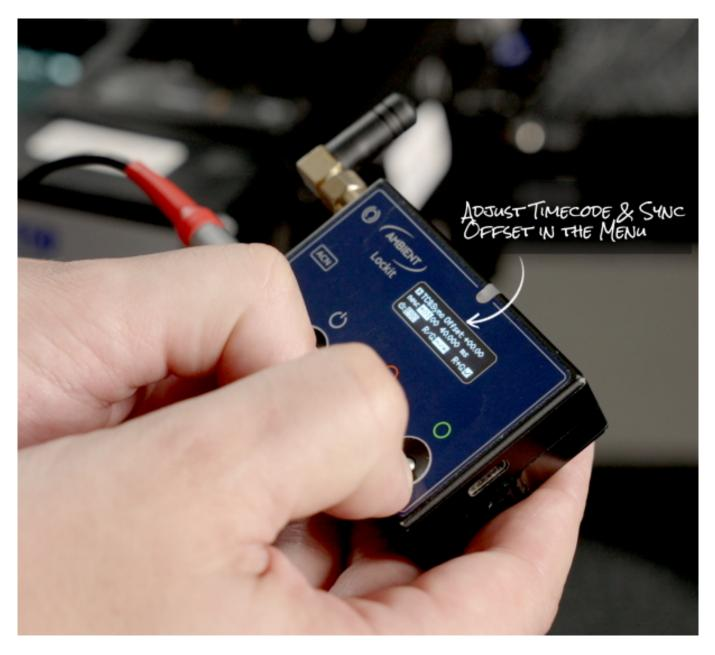
There are cameras that always lag behind for one or more frames even though they get the correct timecode fed in. Use the new Offset feature to solve that issue, which is available for the Lockit, the LockitSlate, and the Lockit+.
