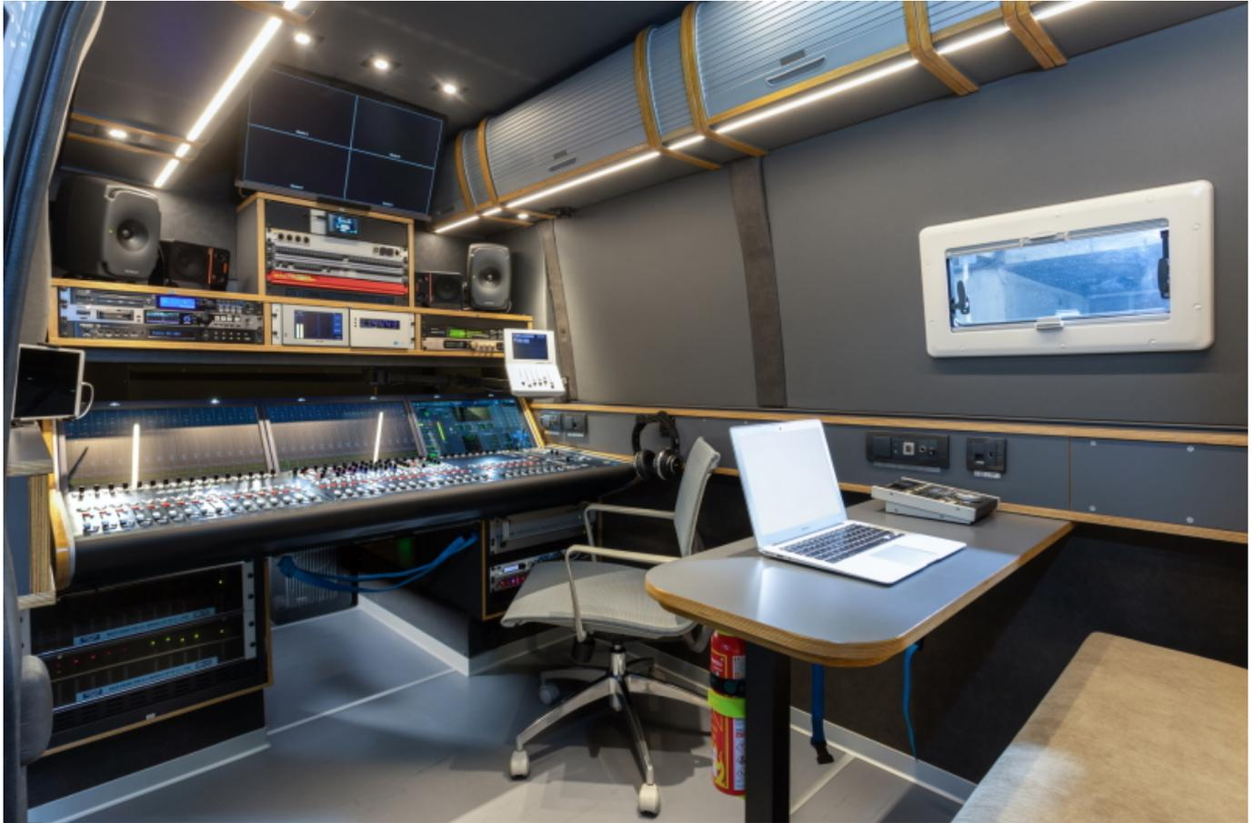
Compact yet flexible and powered by Lawo A\_UHD core technology, mc<sup>2</sup>36 consoles can be sized from 16 to 48 faders and feature intuitive guided workflows, providing 256 DSP channels, 48kHz and 96kHz operation, and 864 channels of I/O capacity. IP-native with support for all relevant standards, it also features redundant power supplies and ST2022-7 'hitless merge' network link redundancy demanded by live broadcast operations.
