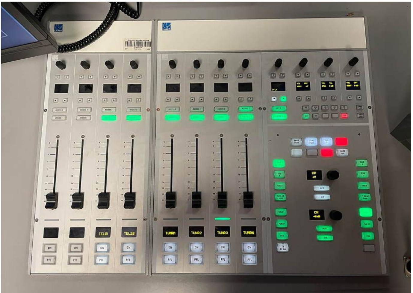
In addition to the ruby mixing consoles, MAP’s radio studios are fitted with Lawo Power Core DSP mixing engines and I/O nodes. These integrate the studios with adjacent voice booths, called “studettes”; the setup then interlinks the studios and studettes with MAP’s large Grand Studio with just the push of a button.
