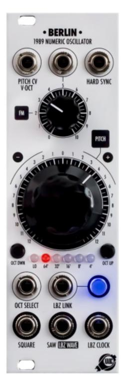
On the surface, Xaoc Devices Berlin is a simple compact VCO offering square and saw waves with hard sync, FM input and octave switching. The most interesting part lies behind the panel and that is the Leibniz Binary Subsystem interface, namely LBZ out and LBZ in. The frontpanel LBZ LINK button and its corresponding gate input switch between the default saw wave and a signal that has been passed
