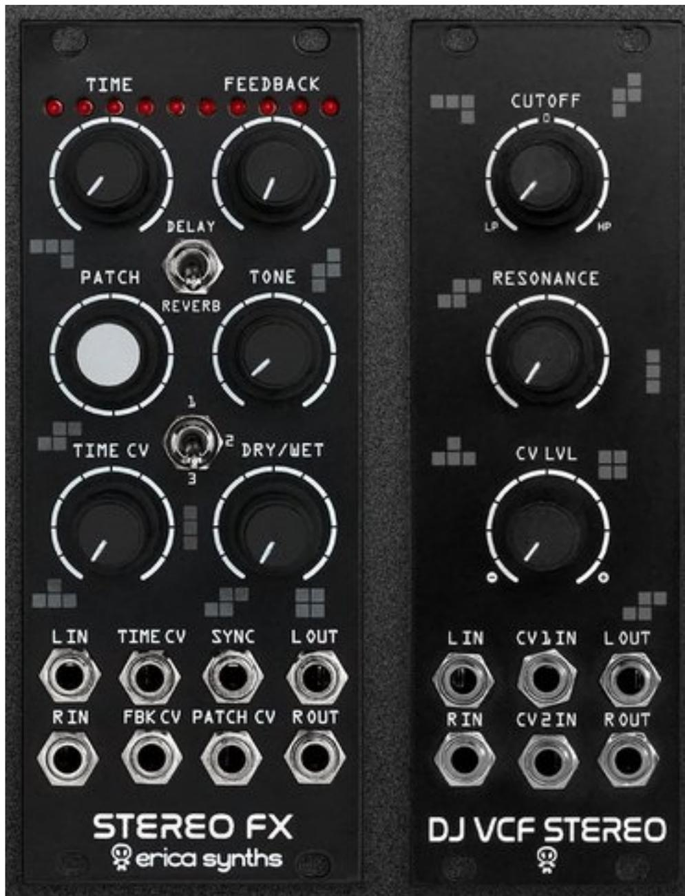
The STEREO FX module brings hi-fi stereo effects into the Erica Synths Drum Series. Based on our new DSP engine, the module provides a wide range of custom delay and reverb effects. CV control over various parameters and the ability to save up to 10 presets will make this module an integral part of any performance rack.
