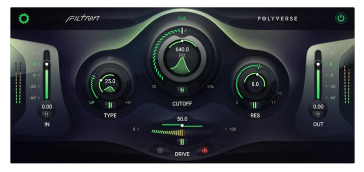
Filtron is a 12dB state variable filter that can smoothly transition between lowpass, bandpass, and highpass. It is capable of self-oscillation with resonance levels that can reach up to 11. Filtron also features a fat sounding internal saturation algorithm and a sizzly post overdrive with two modes to choose from: cold and hot.
