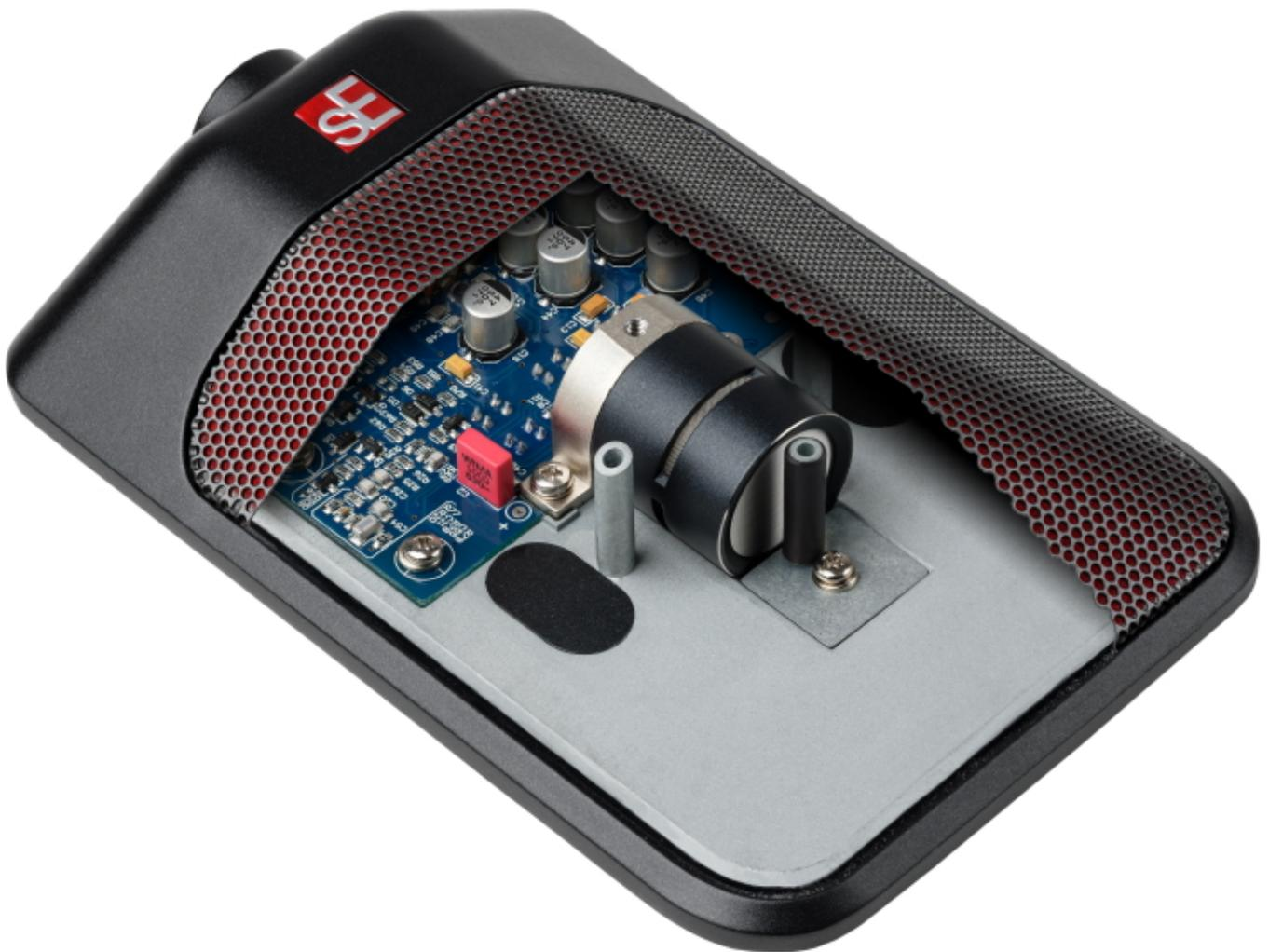
The BL8 utilizes transformerless Class-A circuitry to ensure plentiful headroom without distortion, while its low-noise electronics deliver transparency and clarity. The integrated low-cut filter and optional classic and modern EQ shaping switch make the BL8 an incredibly versatile microphone, excelling at immersive ambience recording, detailed room miking, and it can even be used on acoustic pianos.
