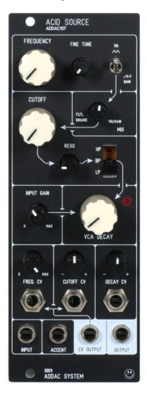
ADDAC System announces its latest Eurorack module, ADDAC107 Acid Source. Acid Source, a compact synth voice incorporating full VCO, VCF and VCA functionality, forays deep into acid sonic territory with classic 'squelchy' sounds - all of which may be shaped using its built-in low-pass, band-pass and high-pass filters. Whether being used for a plucky bass line, a squelchy lead synth line or scratchy percussion,
