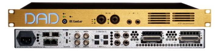
AX Center is a dedicated Thunderbolt modular audio interface with dual Mic and Instrument inputs, dual Headphones and Monitors outputs built-in PRO|MON monitor control with speaker EQ and two slots for DAD expansion cards. It comes with 256 Thunderbolt 3 channels, 256 Dante I/O channels, up to 192 MADI I/O channels and 16 ADAT channels, as well as onboard summing and processing.
