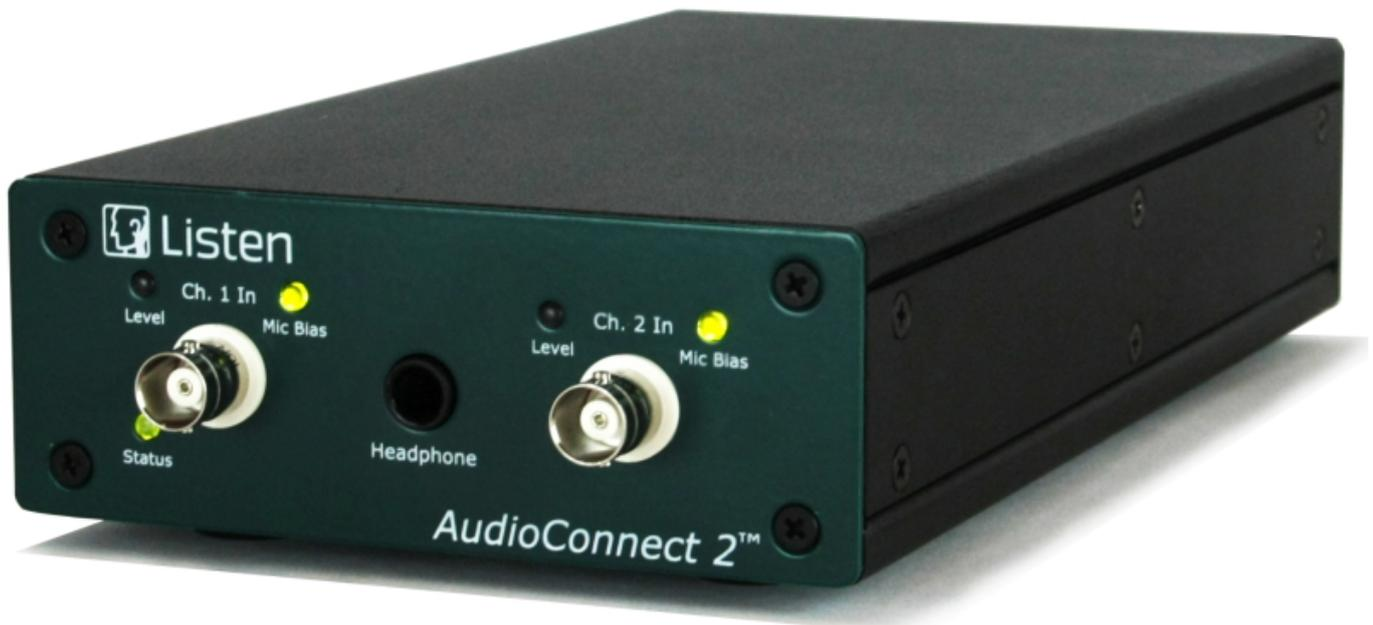
AudioConnect 2, Listen's new compact and high resolution two-channel audio interface is designed for measurements anywhere from the production line to out in the field, and is particularly suitable for headphone testing and in-car measurements. It features 2 input channels with a sampling rate up to 192 kHz, microphone power, TEDS support, a low-noise headphone amplifier, and two line outputs. It can be powered via a laptop's USB-C for portability and for field measurements.
