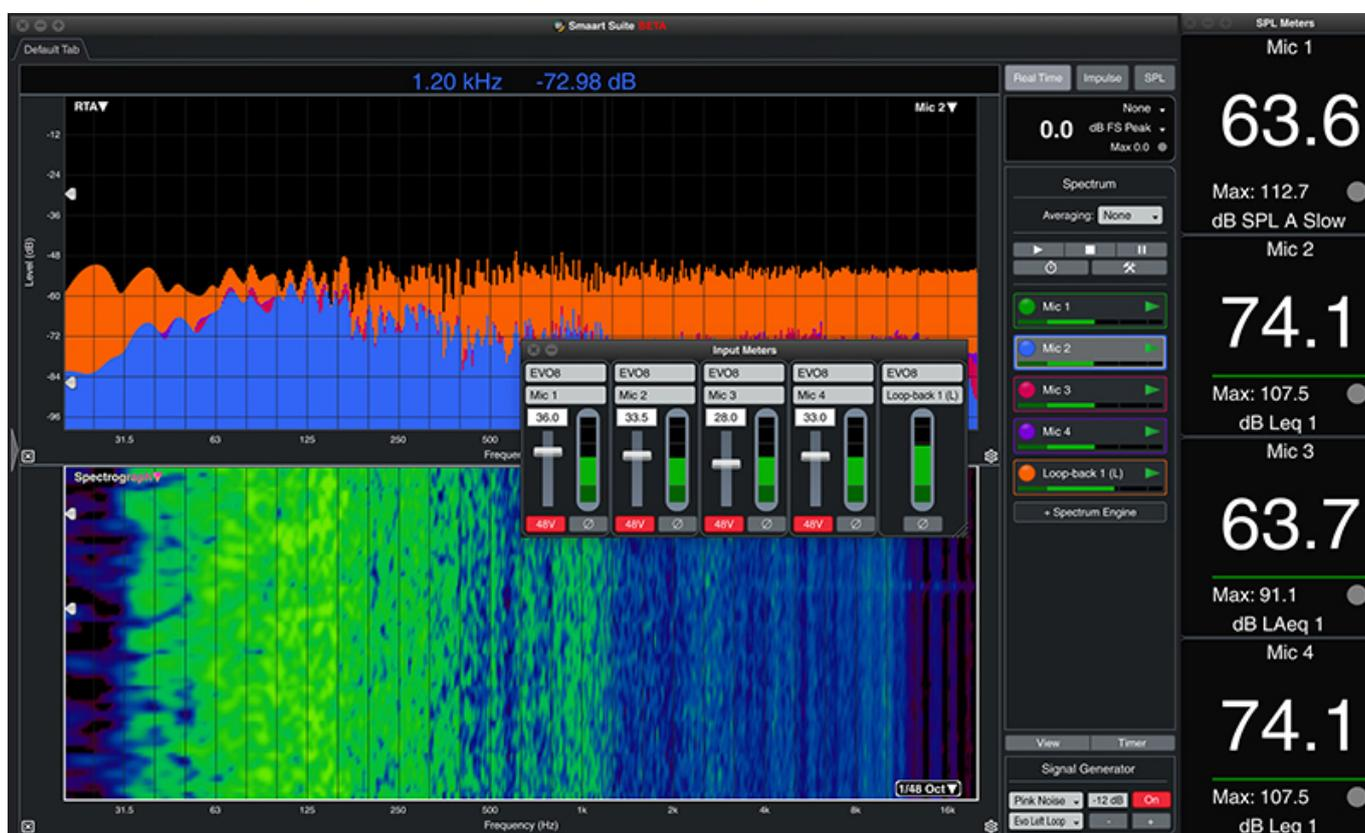
Rational Acoustics LLC and Audient Ltd. announce the upcoming integration between Smart v9 and the EVO line of audio interfaces. The Smart 9.1 update, scheduled to be released in mid-December integrates the controls for phantom power and gain for Audient's EVO devices - EVO 4, 8, and 16 - directly from within the Smart interface. Additionally, gain tracking may be enabled to allow for automatic decibel offset recalculation for calibrated inputs.
