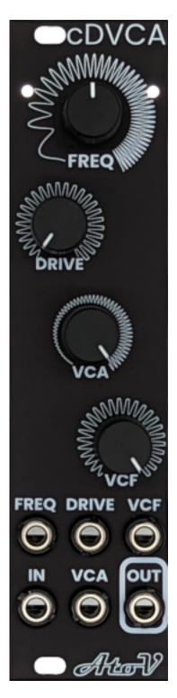
cDVCA or class-D VCA is a new kind of VCA based on an entirely novel concept that is inspired from class-D amplification technology allowing for never heard before waveshaping. The input signal is turned into an ultrasonic PWM signal. The PWM is
