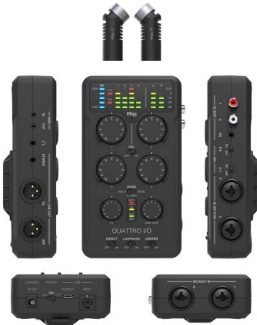
In Stereo mode, iRig Pro Quattro I/O mixes all sources down to stereo for streaming or recording. Monitoring is easy thanks to a dedicated headphone output with independent volume control and direct monitoring. Mono mode extends compatibility for streaming to social media. A Loopback feature lets users easily duet with favorite videos, plus iRig Pro Quattro I/O can also keep the device under charge for long streaming sessions, using its power supply unit.
