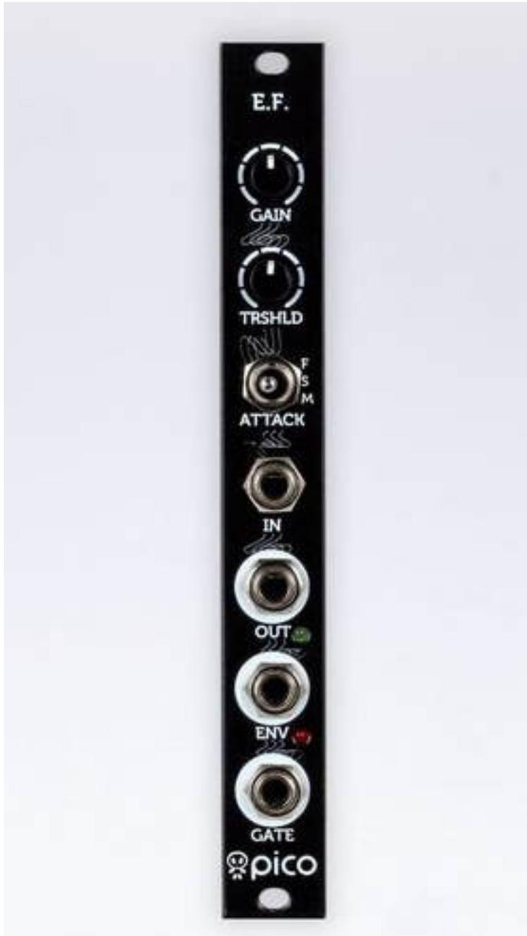
Pico EF is Erica Synths take on envelope follower module in 3hp! Pico EF features a preamp with +40dB gain (enough to boost even guitar and dynamic microphone signals for use in a modular system), envelope output with adjustable attack time and a gate output with adjustable threshold. The Pico EF can be used as a preamp, overdrive unit or for controlling VCFs with audio signal, or to use with external instruments to control your modular system in other creative and experimental applications.
