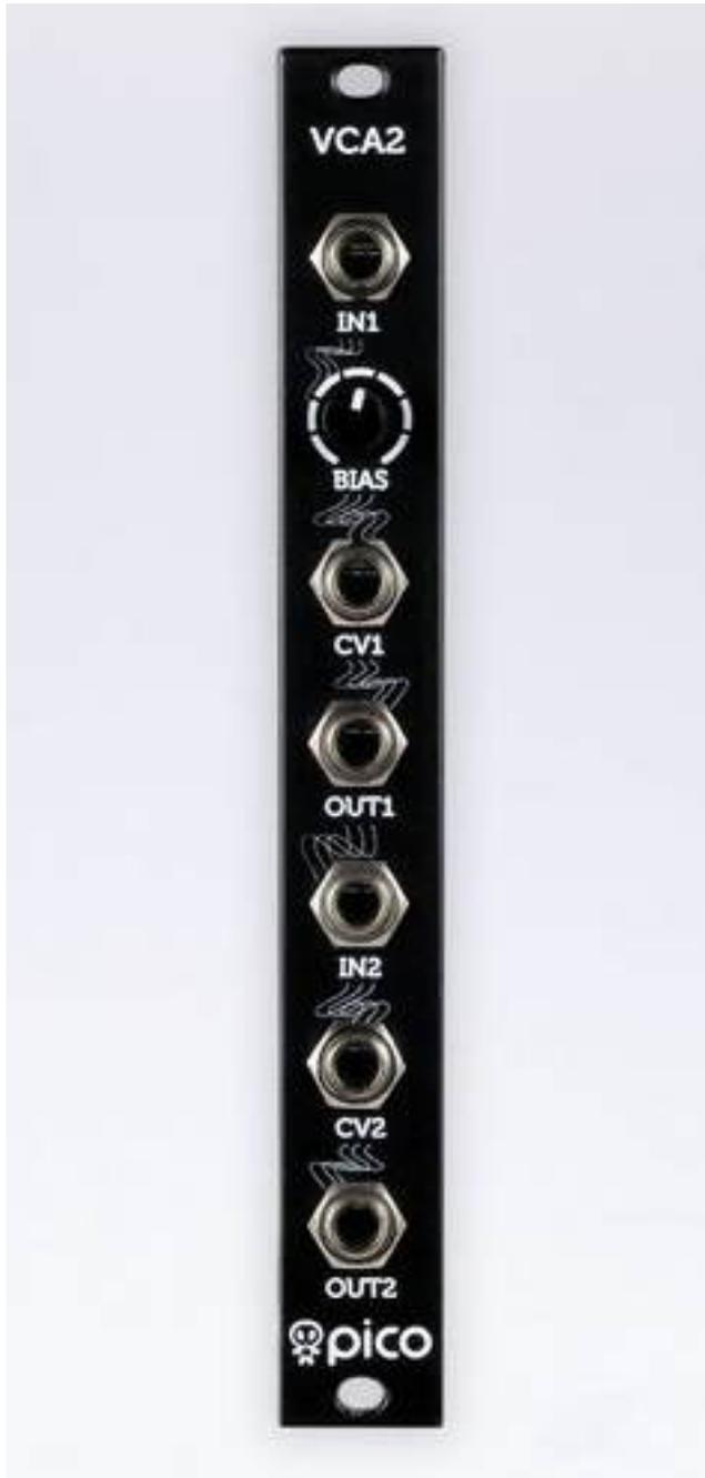
The Erica Synths Pico VCA2 is a compact voltage controlled amplifier module, based on reliable AS3330 chip. It features two independent channels, and the first one comes with the manual offset adjustment, useful for full span vibrato effects. Audio and CV inputs of the first VCA are normalised to the second one, so the module can also be used as a buffered audio splitter. VCAs are DC coupled, and they can be used for controlling amplitude of control voltage signals.
