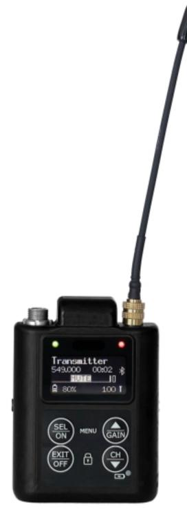
Wisycom announces the immediate availability of its new MTP61 Miniature Multiband Transmitter, the latest addition to its Symphony product line. The smallest and lightest multiband bodypack transmitter on the market, the MTP61 has the widest tuning range currently available (470 to 1260MHz). In support of the official launch of the transmitter, Wisycom is also releasing its new LBC61 4+4 Mittwoch, 14. Juni 2023 20:01
