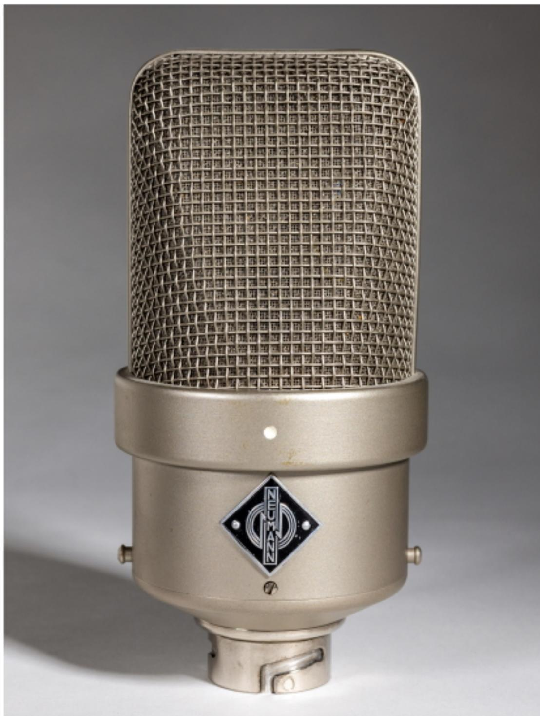
The Neumann M 50, which was introduced in 1950, was instrumental in the development of the Decca tree recording technique. Its open-mesh head basket houses a small-diaphragm capsule flush-mounted in a small sphere, and its unique acoustic properties are ideally suited to orchestral recordings.
