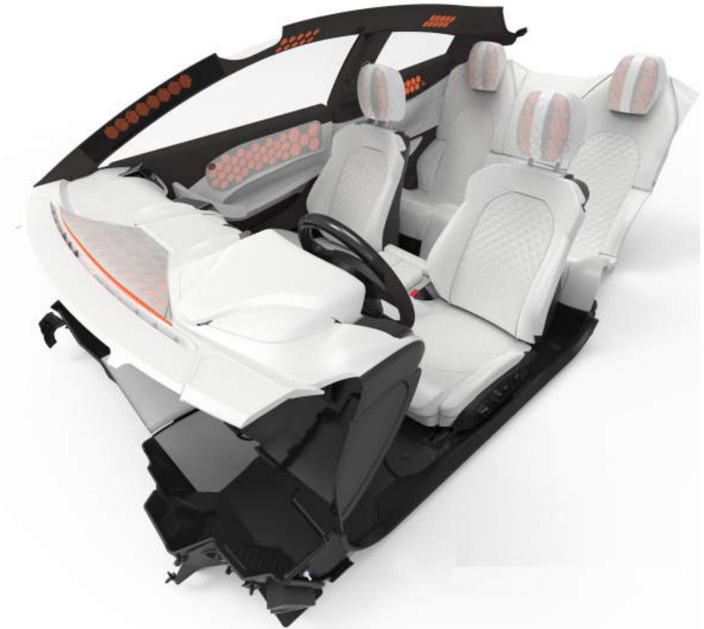
Warwick Acoustics' ElectroAcoustic Panels bring significant whole vehicle system benefits compared to the use of conventional audio technology. Like-for-like, ElectroAcoustic Panels are up to 75% lighter, consume up to 75% less power and offer significant interior design and packaging freedom.
